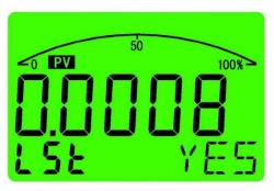
menu area displays "LSt", select the desired operation through the "S" and "Z" keys, and the prompt area displays accordingly:
