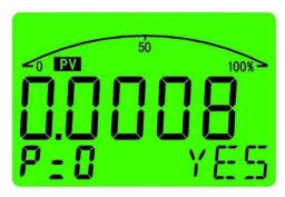
in the right figure, the menu area displays "P=0", through the "S" key and "Z" key to select the desired operation, the prompt area will display correspondingly:
