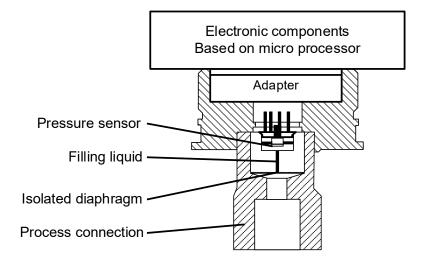
Pressure transmitter includes two functional units:
