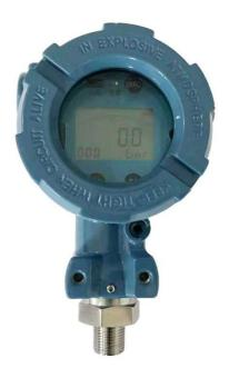
DR3704 digital pressure gauge from Fandesensor now offers data-logging capability with SD card to facilitate data logging, users can transfer the stored data to a PC or laptop in CSV file format, where they will see a time and date stamp against recorded pressures. such data sets are particularly useful for trend analysis or if there is a specific system event that requires investigation. It offers the continuous monitoring of oil, gas, water and other pressure media.
